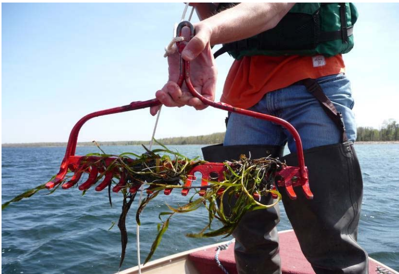
Figure 1. Double-sided, weighted garden rake
